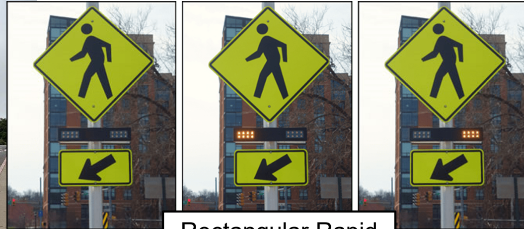
Rectangular Rapid Flashing Beacon
