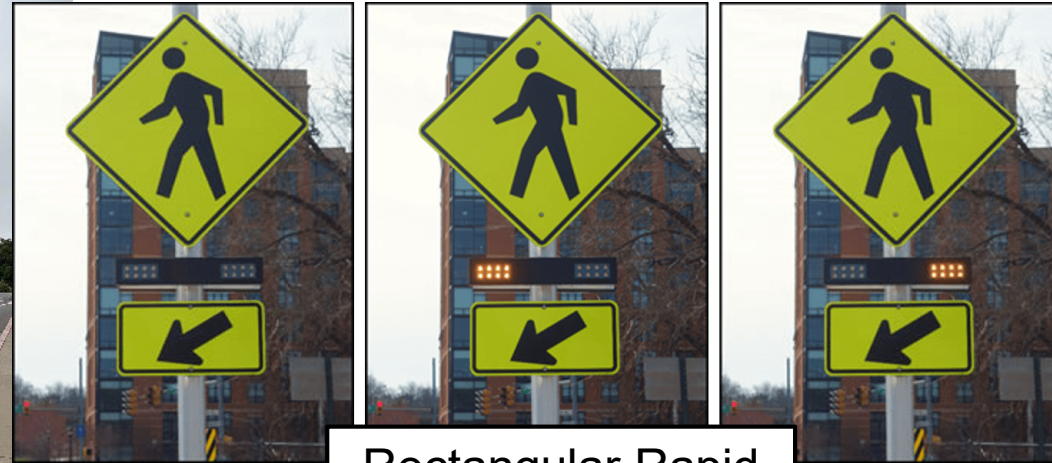
Rectangular Rapid Flashing Beacon
