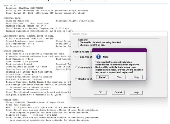
When the ALOHA program was prompted to run the vapor cloud explosion model the result was that such an explosion was not a possibility:
