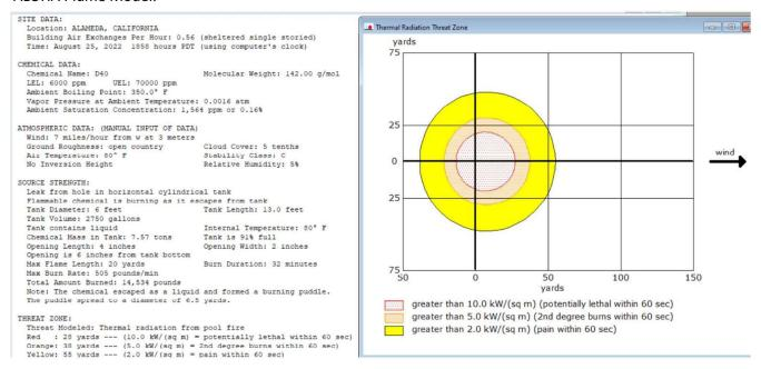
The above plume model was based on the highly un-probable scenario that something like a forklift tine pierced the double walled tank and the cinder block secondary containment berm was also damaged; such that the leaking fuel could form a puddle around the tank – and then somehow the pool of fuel found an ignition source and caught fire.
