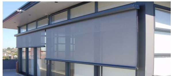
Exterior roller screens.
