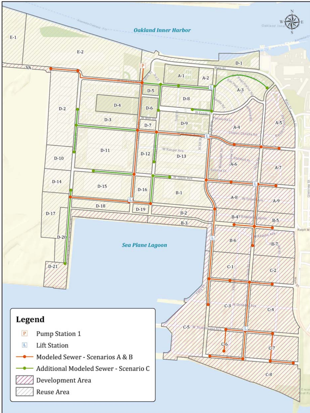
Figure 1: Alameda Point Proposed Sewer System - Modeled Network
