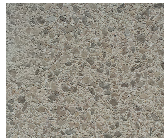
CONCRETE PAVING TYPE #1 NATURAL GRAY HEAVY SANDBLAST
