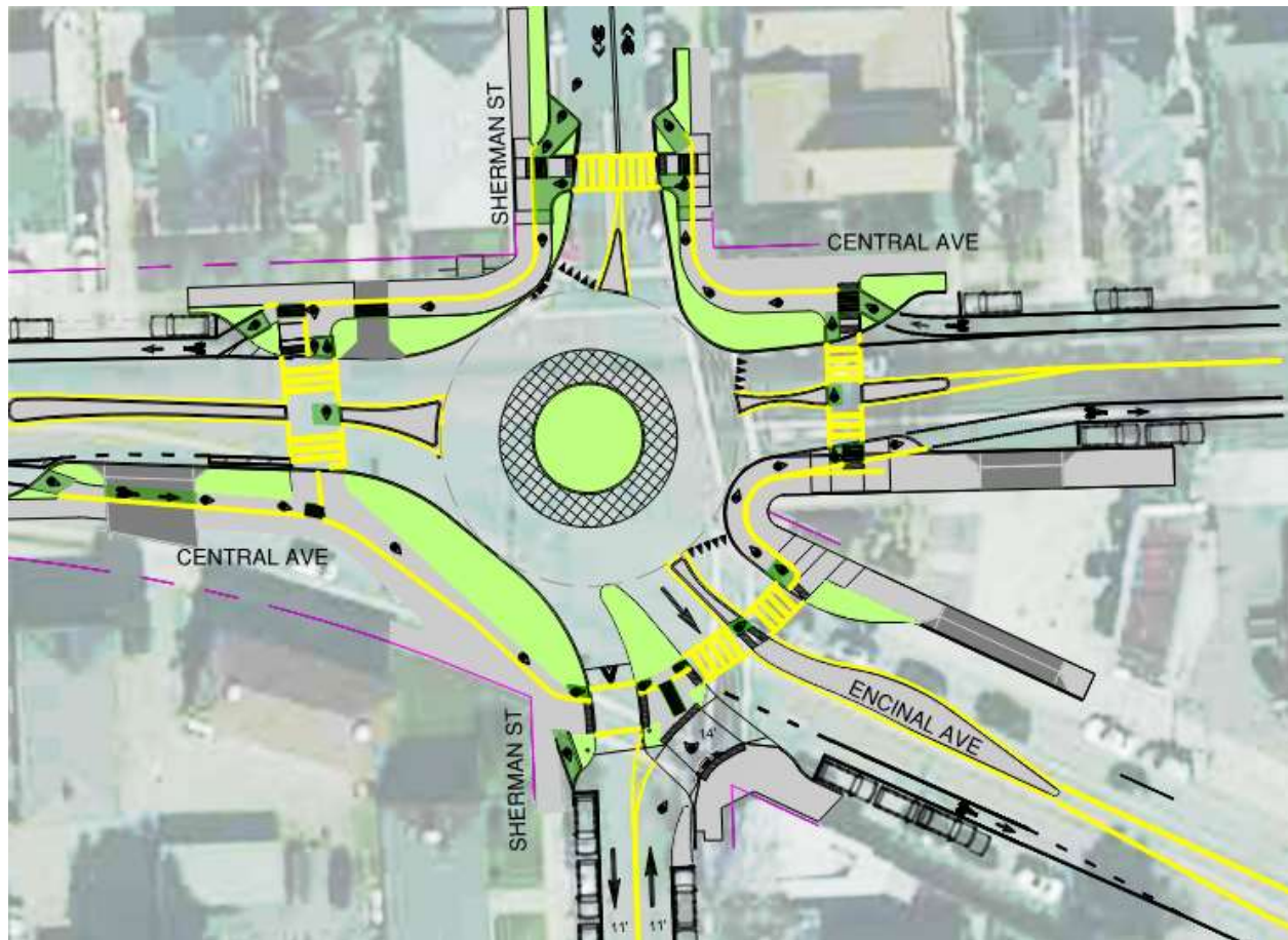
Figure 5: Recommended “Slip Lane” alternative
