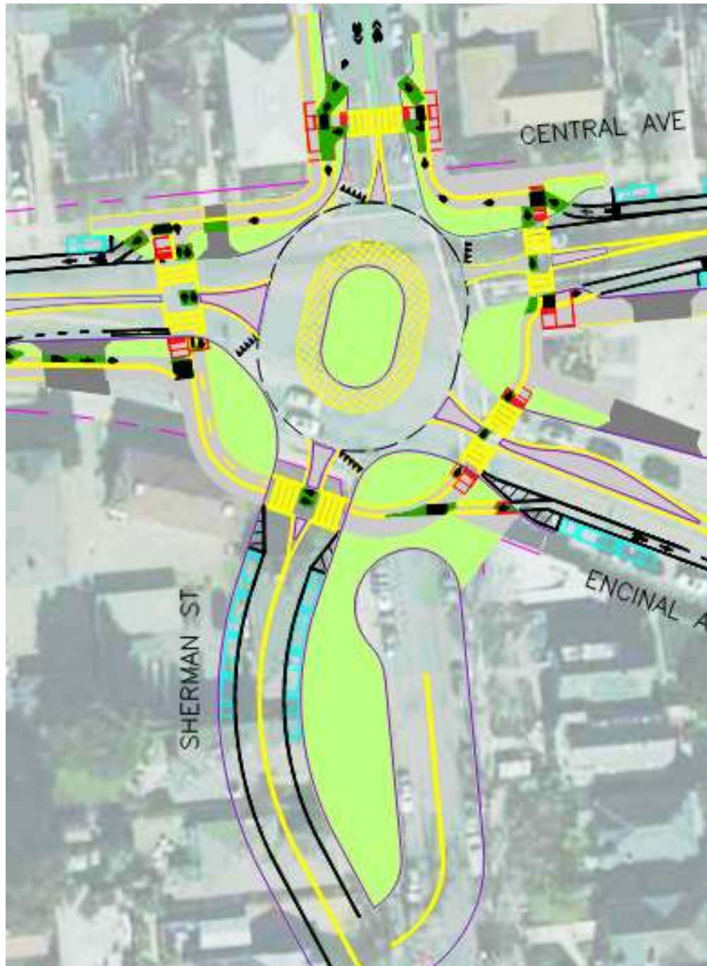
Figure 4: Fully functional roundabout meeting all design guidance
