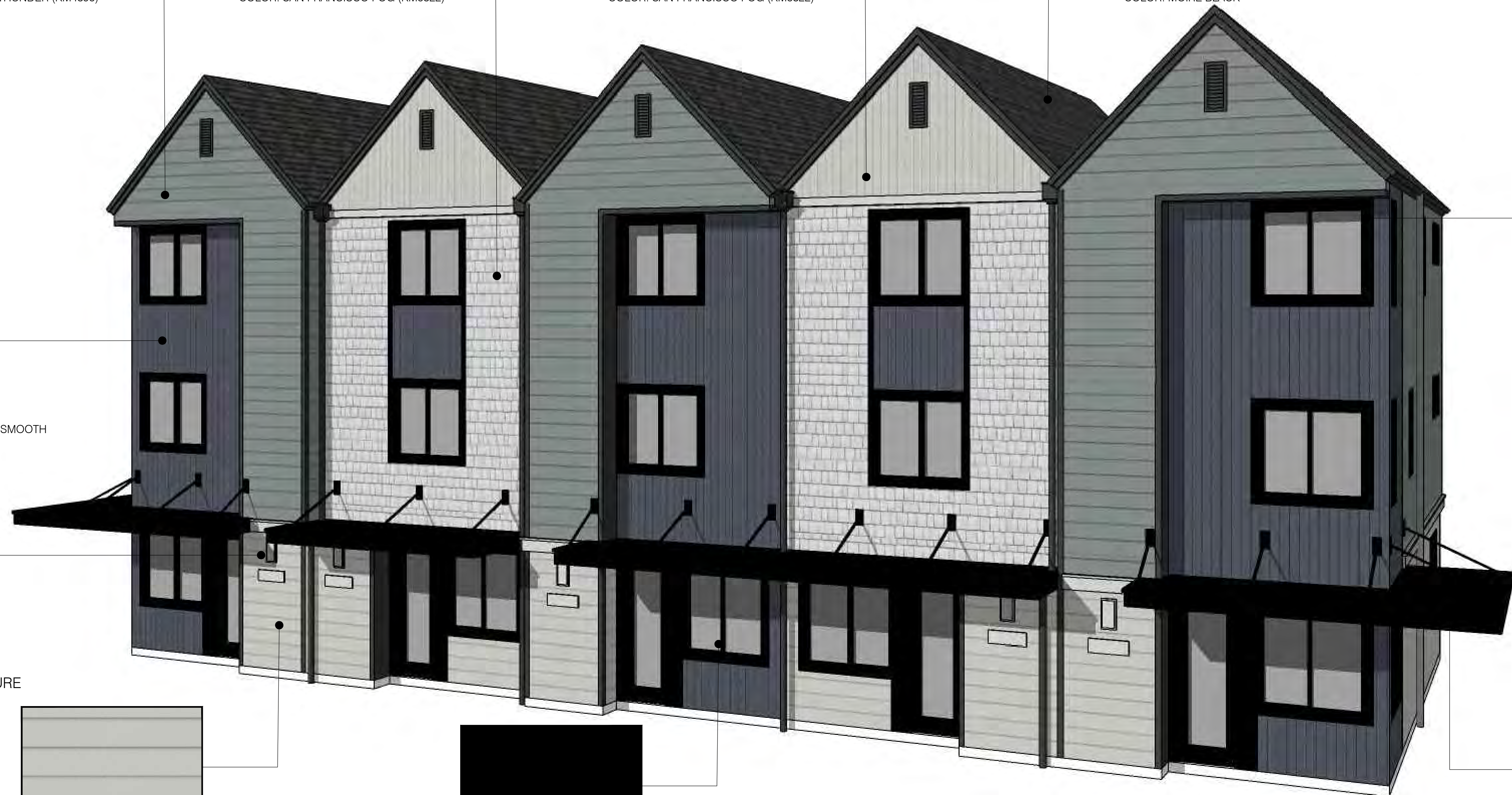
SIDING 1 HORIZONTAL CEMENT BOARD SIDING - SMOOTH PAINT: KELLY MOORE COLOR: DISTANT THUNDER (KM4895)
