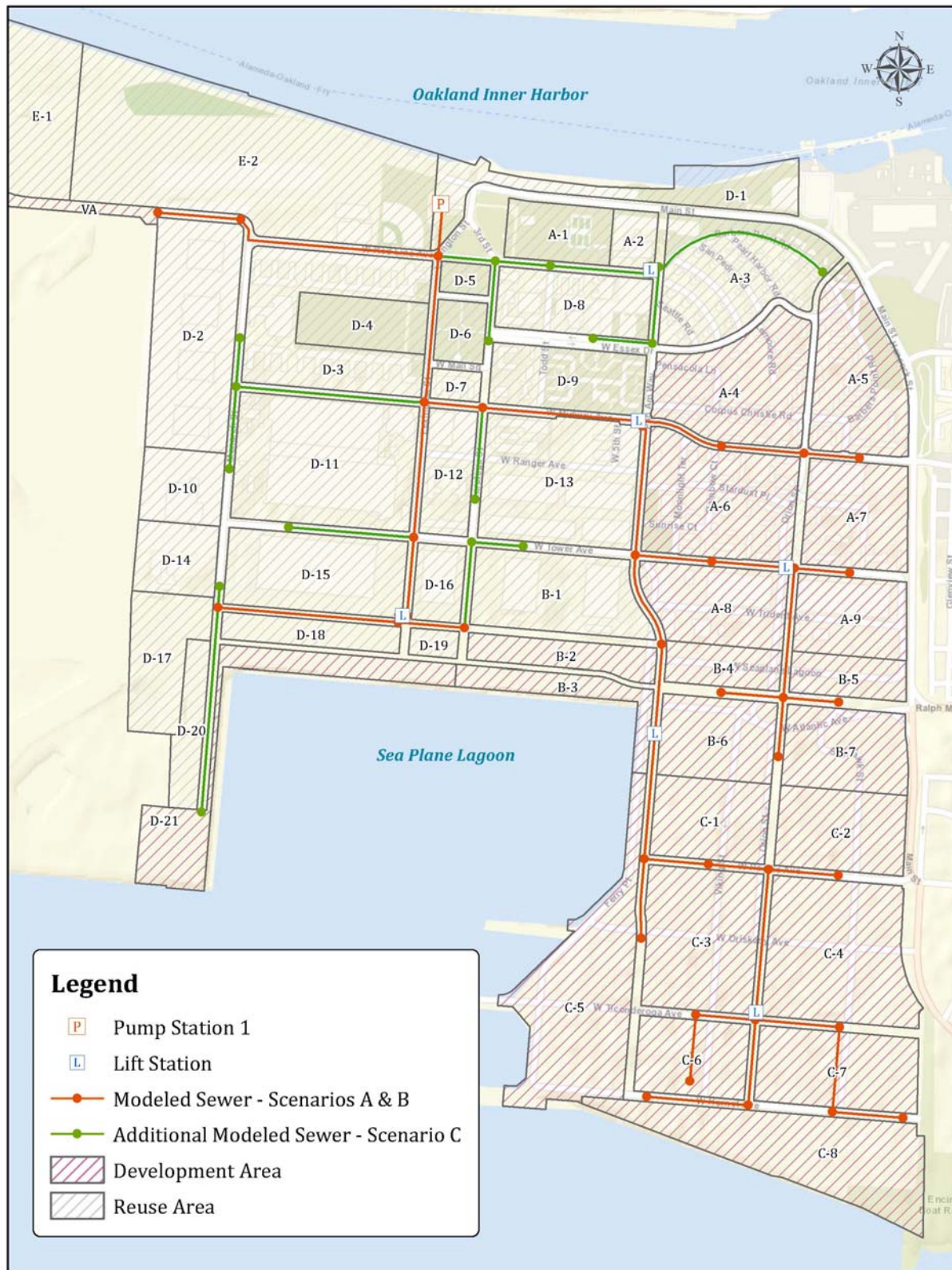
Figure 1: Alameda Point Proposed Sewer System - Modeled Network
