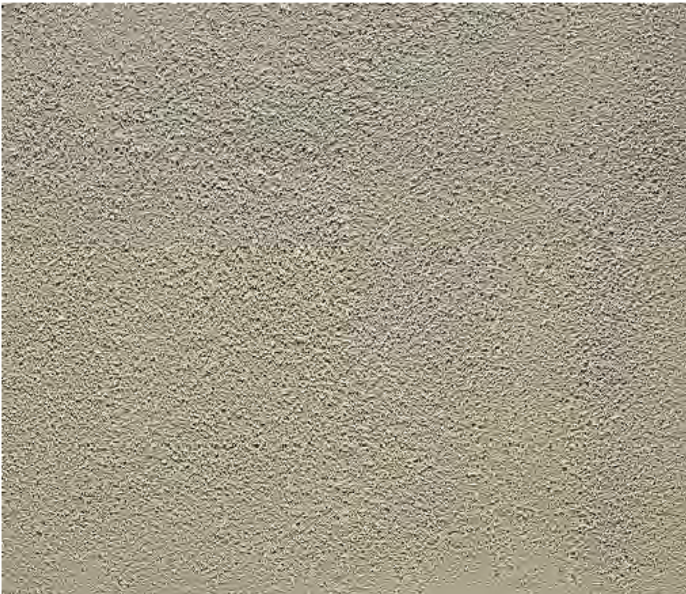
SAND FINISH STUCCO (SEE ELEVATIONS FOR COLORS)
