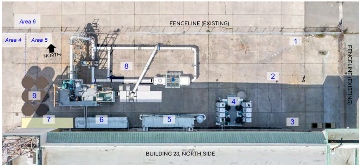
Figure 6: detailed site plan for operations area (Area 5), corresponding with Table 2.
