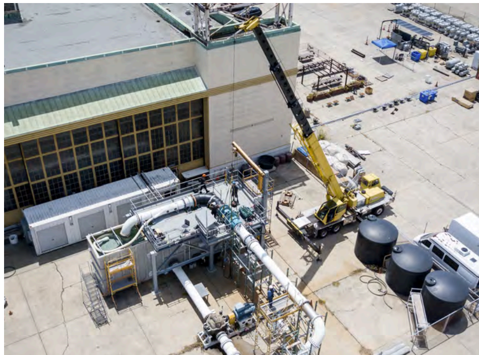
Figure 11: Occasionally, large lifting equipment is required for the placement of test components into the hydraulic test facility. This is one of the reasons why this equipment is located outdoors.
