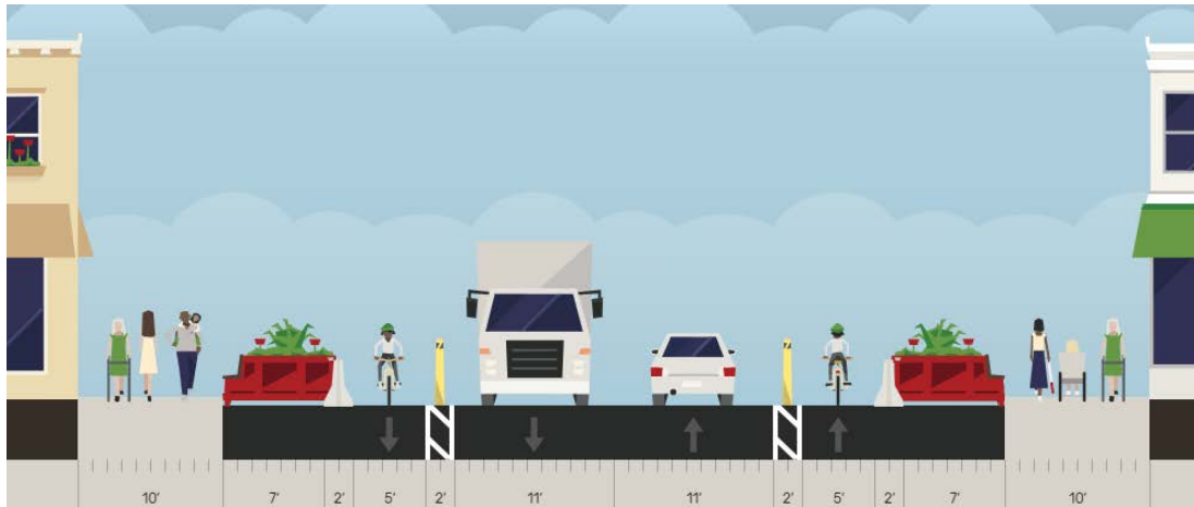
Figure 1: Standard cross section of the draft recommended striping plan in areas where parklets are located in front of businesses.
