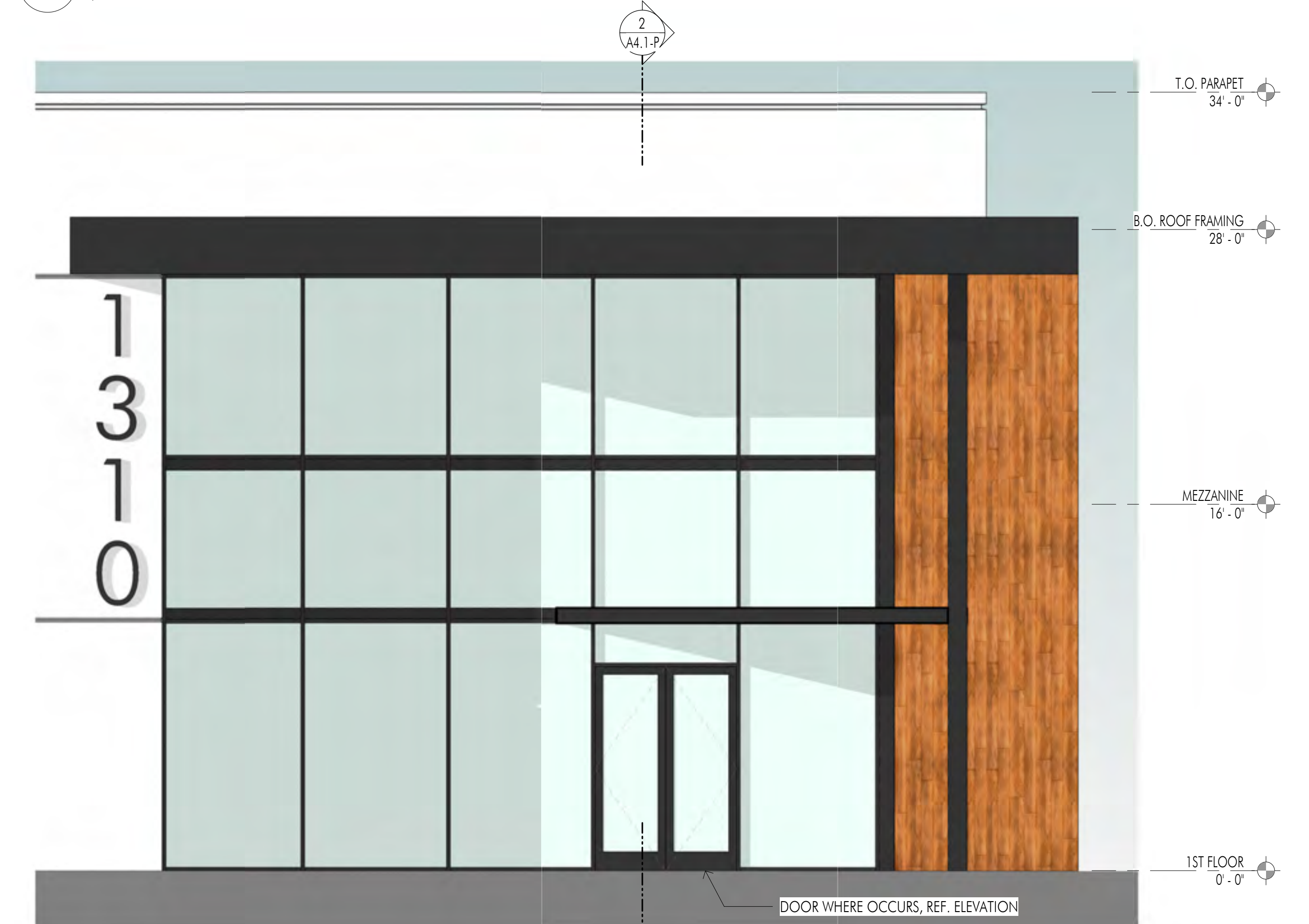
1 TYP. ENLARGED NORTH-FACING ENTRY ELEVATION 1/4" = 1'-0"
