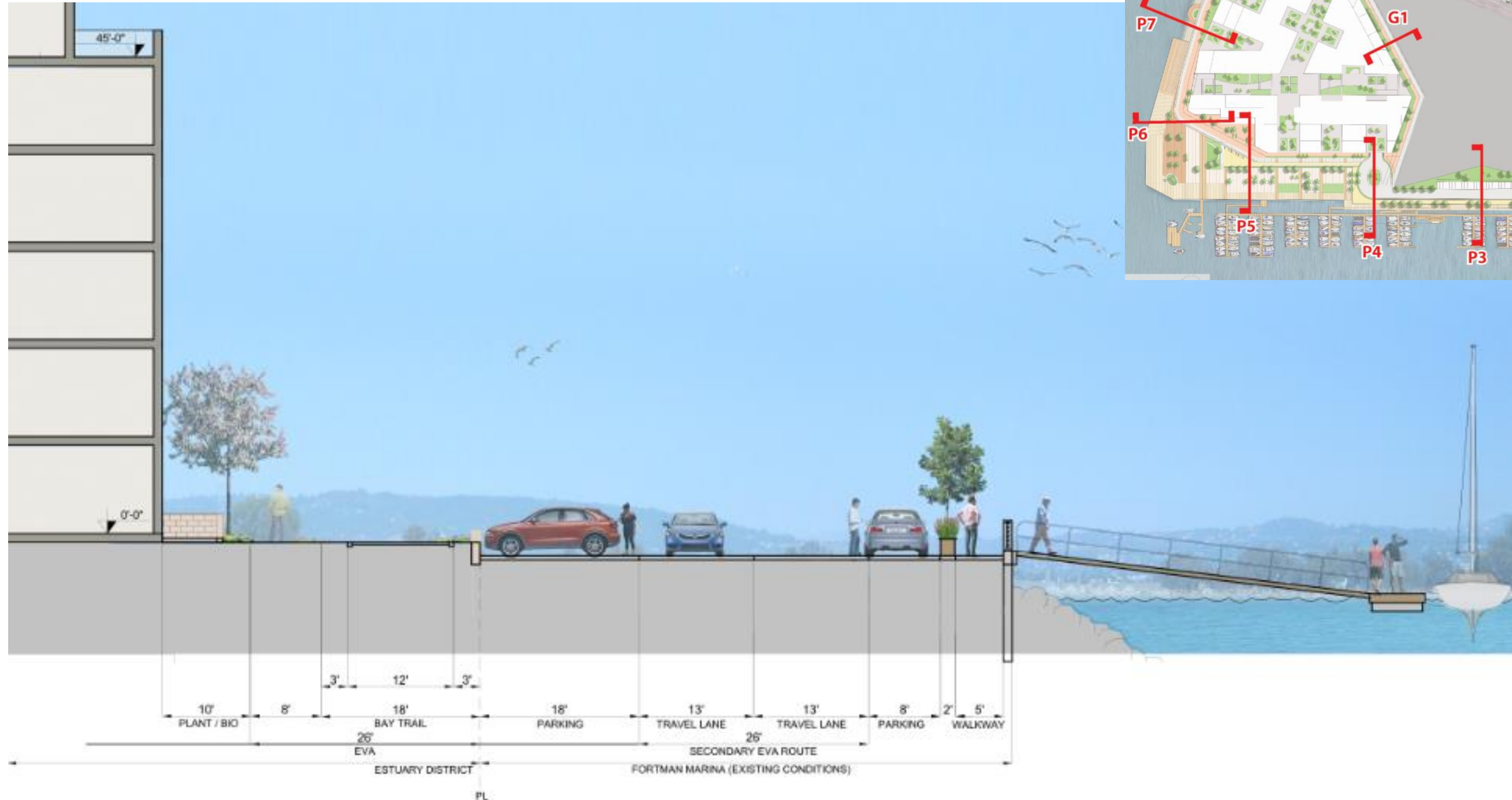
FIGURE 3.13 ILLUSTRATIVE CROSS SECTION F1: BAY TRAIL AND EAST EDGE OF THE ESTUARY DISTRICT (VIEW LOOKING NORTH)
