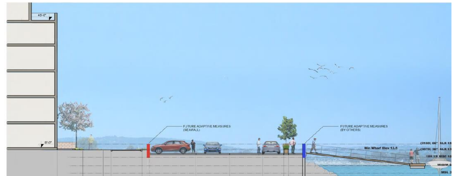
FIGURE 2.8 ADAPTIVE MEASURE AT FORTMAN EDGE (SECTION F1), SHOWING PRIMARY MEASURE IS A SEAWALL AT WATER'S EDGE (BY OTHERS). SECONDARY TREATMENT OF A SEAWALL AT THE ENCINAL/FORTMAN PROPERTY EDGE IN THE EVENT IMPROVEMENTS CANNOT BE MADE ON FORTMAN PROPERTY
