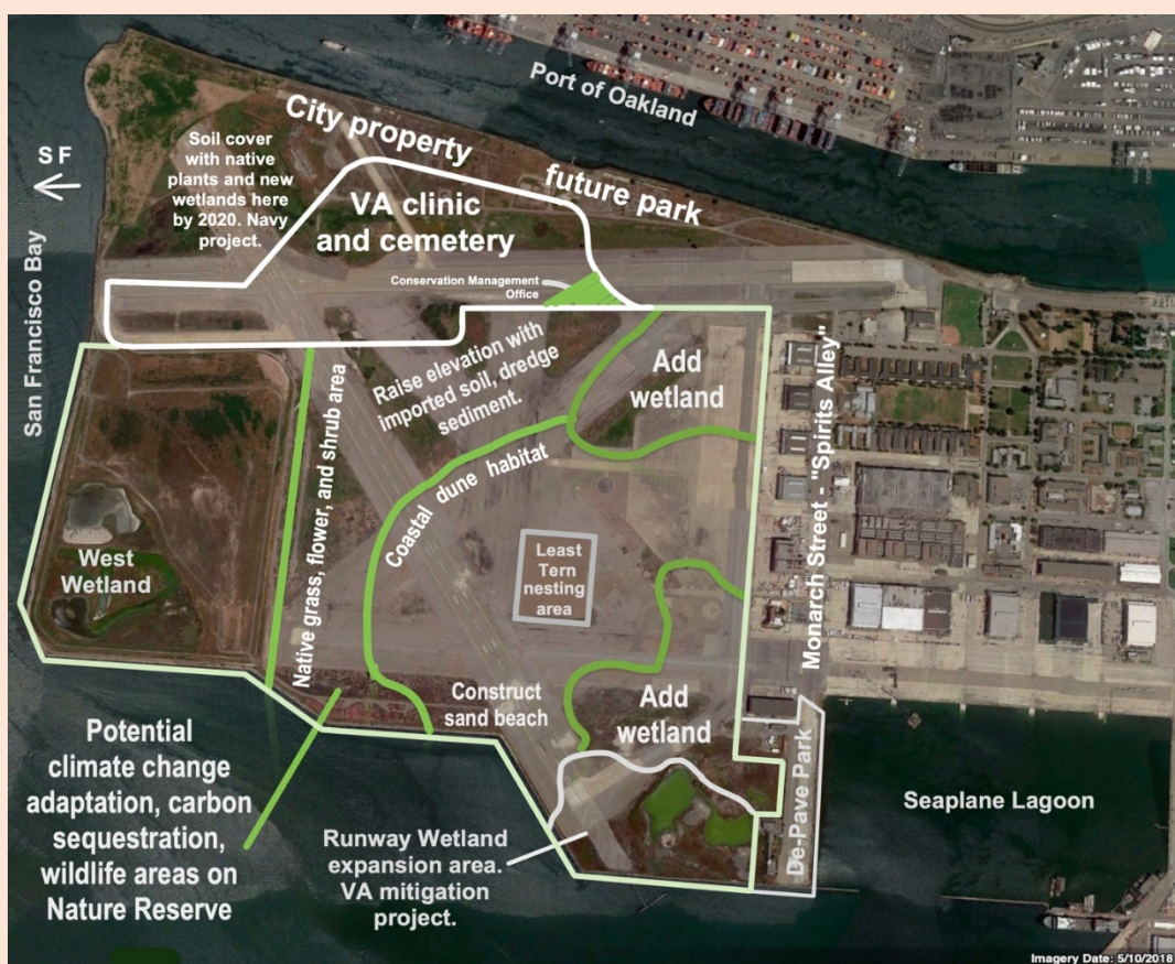
Figure 4-12. Conceptual map for land exterior to the perimeter levee at Alameda Point.
