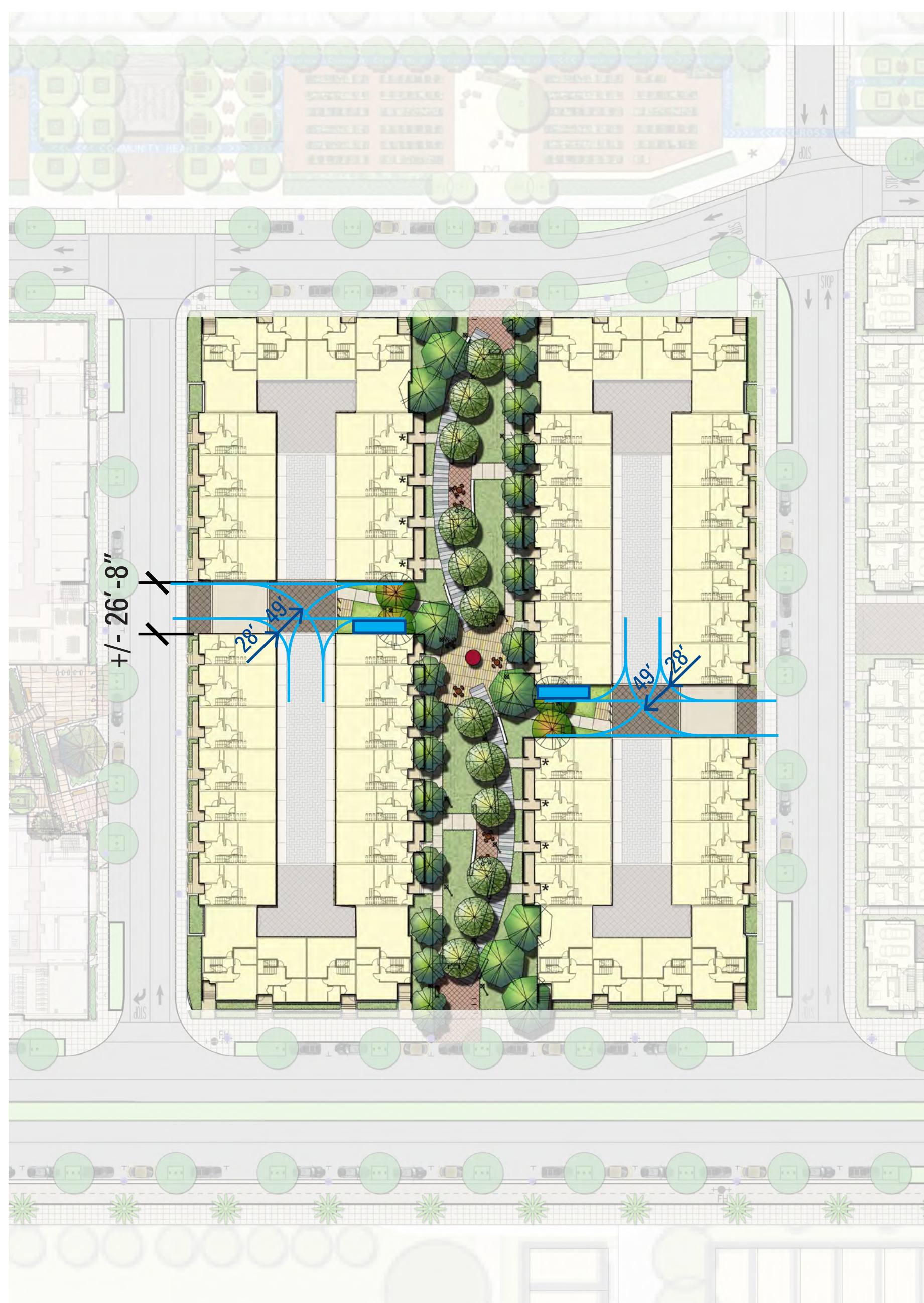
OPTION 2: CONSOLIDATED COLLECTION @ COURTYARD A WOOD SLAT SCREENED, CONSOLIDATED WASTE COLLECTION ENCLOSURE IS PROVIDED ACROSS FROM EACH PARKING COURTYARD ENTRY
