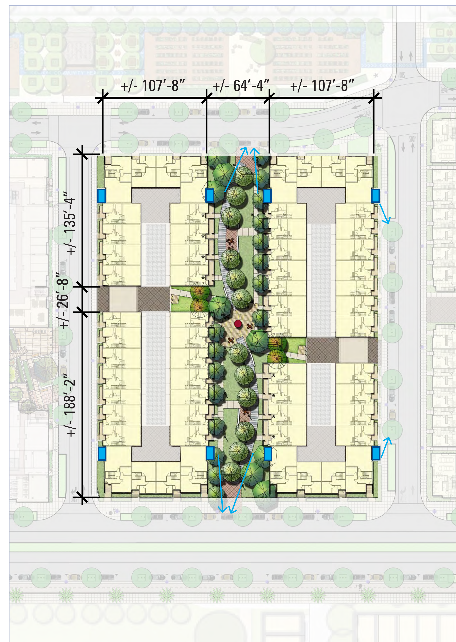
OPTION 3: CONSOLIDATED COLLECTION @ PERIMETER A WOOD SLAT SCREENED, CONSOLIDATED WASTE COLLECTION ENCLOSURE IS PROVIDED ALONGSIDE UTILITY SHEDS SERVING THE BLOCK. DURING WEEKLY COLLECTIONS, WASTE COLLECTION BINS ARE ROLLED OUT TO THE STREET FOR PICKUP
