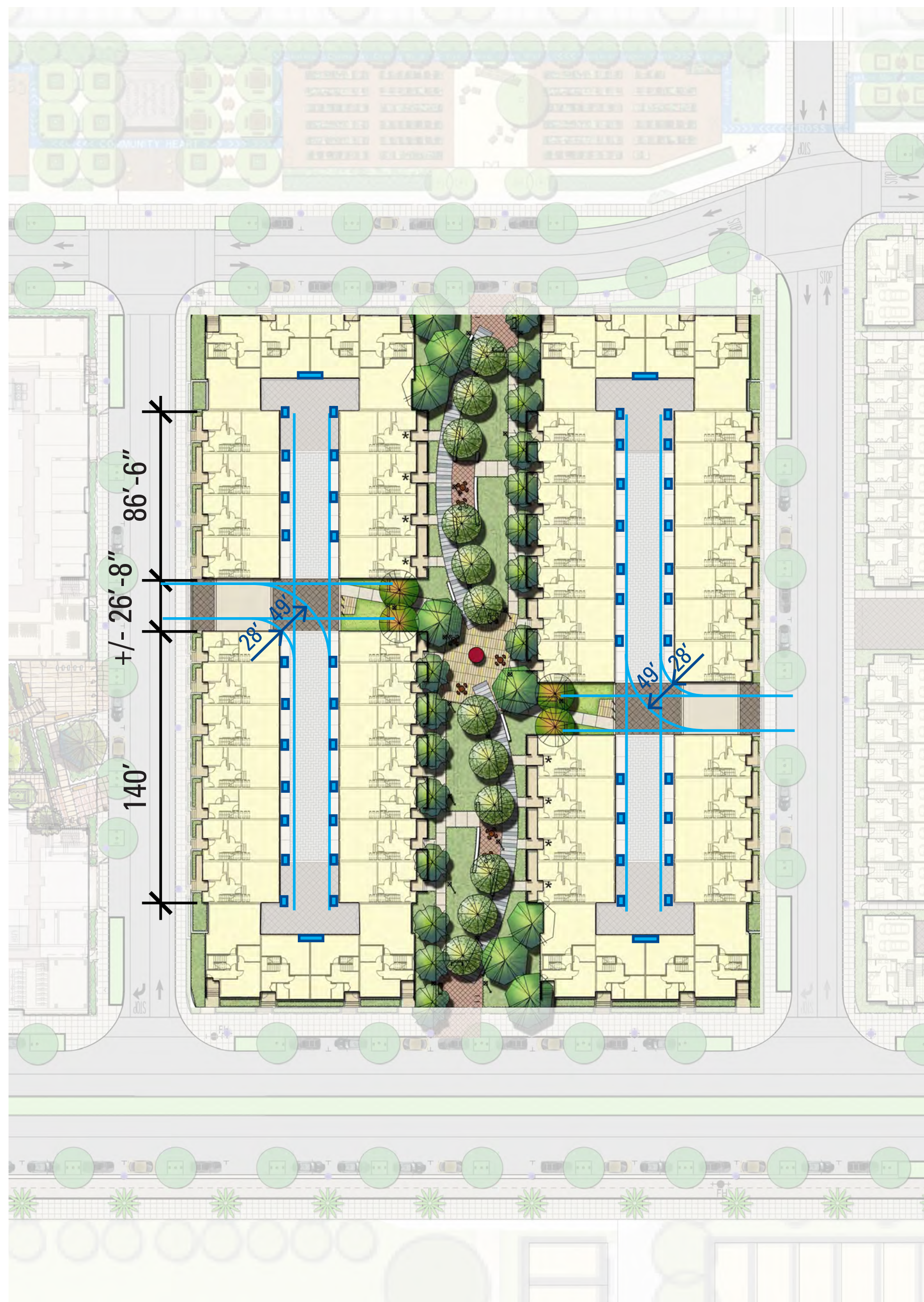
OPTION 1: INDIVIDUAL UNIT COLLECTION @ COURTYARD INDIVIDUAL WASTE BINS ARE BROUGHT OUT ALONG UNIT GARAGES, WITH CONSOLIDATED TRASH BIN AREA FOR BLOCK END UNITS
