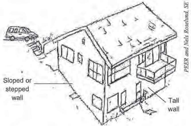
Figure 24 - Hillside homes with sloped and tall walls or posts require special engineering.
