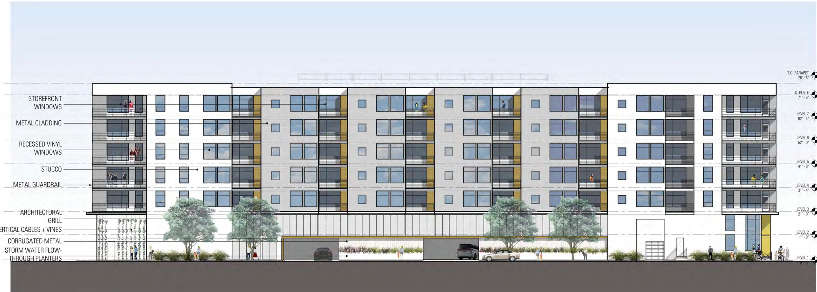
EXTERIOR ELEVATION - NORTH
