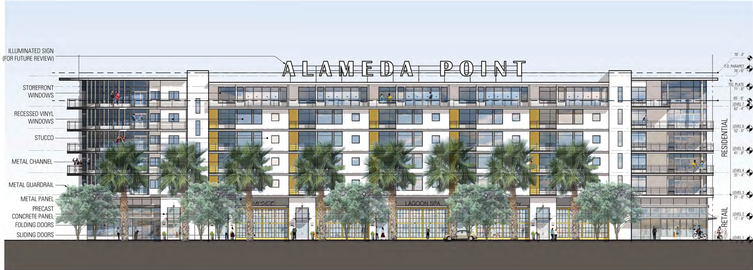
EXTERIOR ELEVATION - SOUTH
