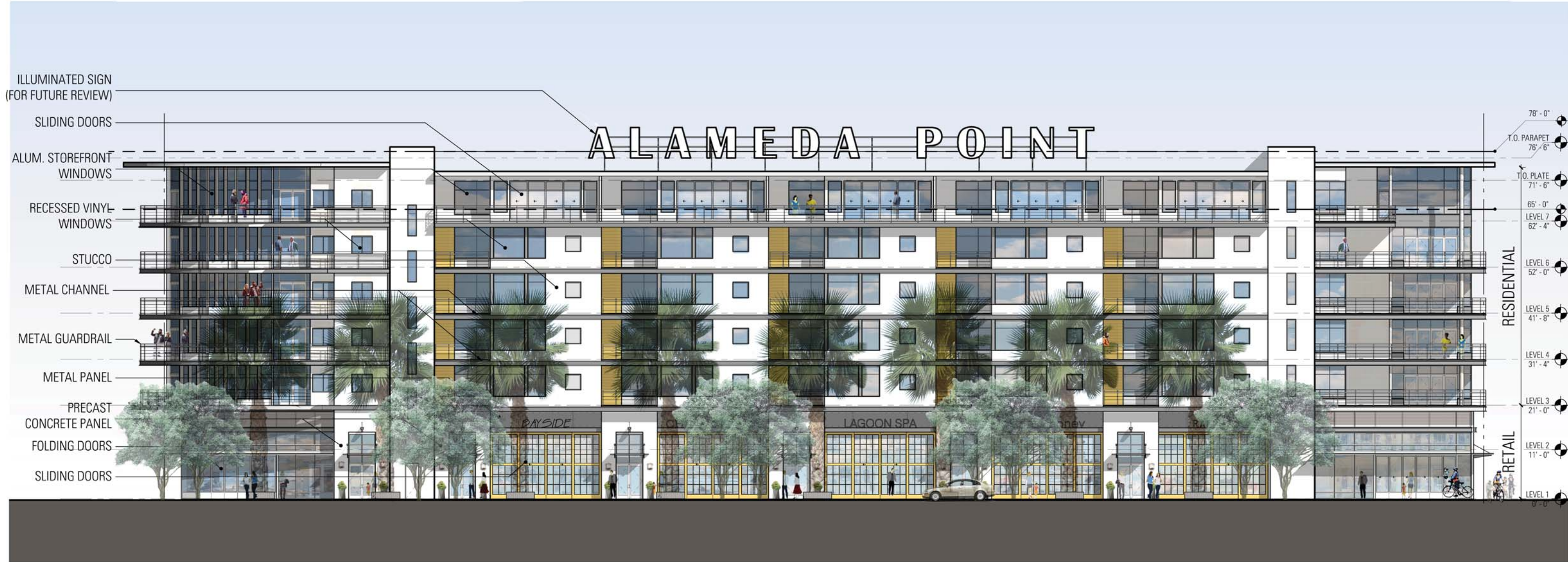
EXTERIOR ELEVATION - SOUTH
