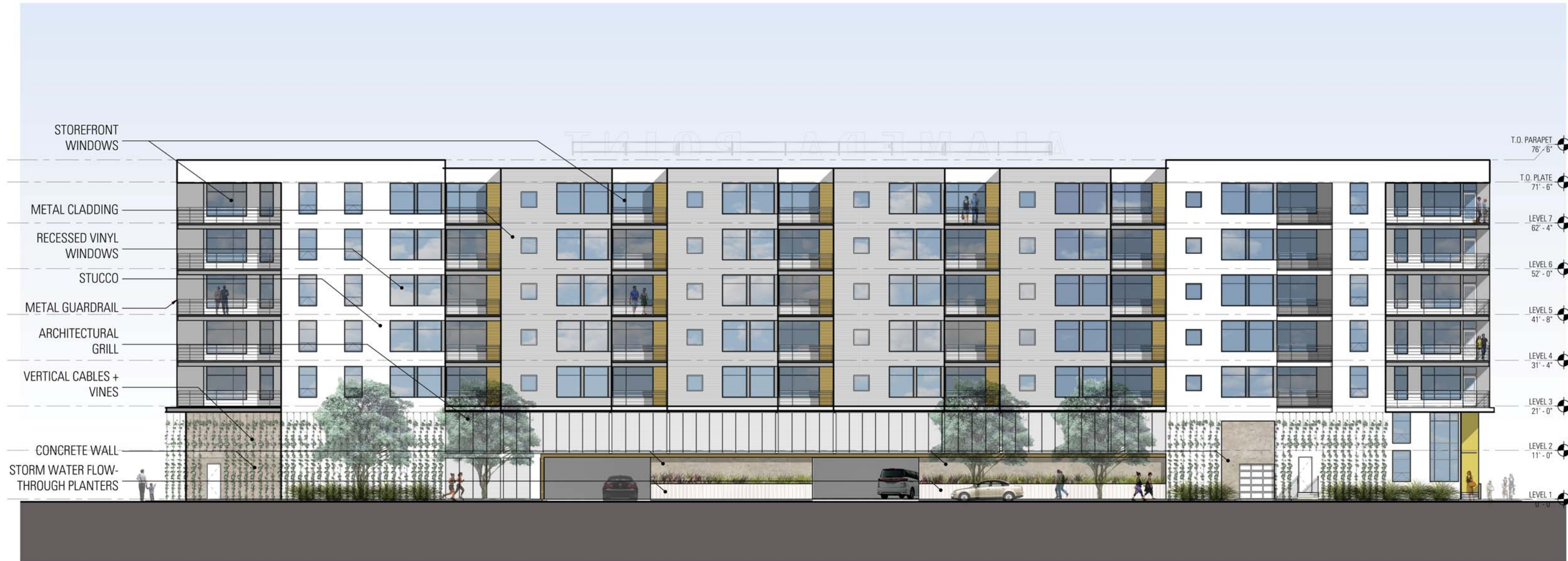
EXTERIOR ELEVATION - NORTH
