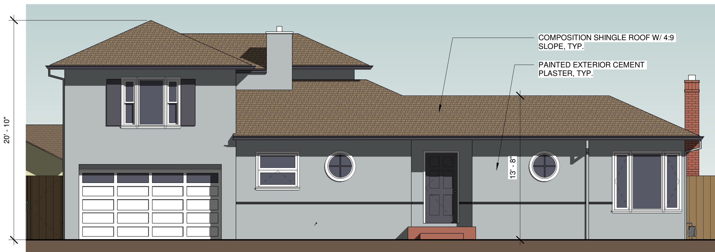
1 EXISTING SOUTH EXTERIOR ELEVATION 3/16" = 1'-0"
