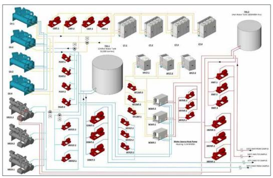
Design 3 - Hydronic System Single Line Diagram
