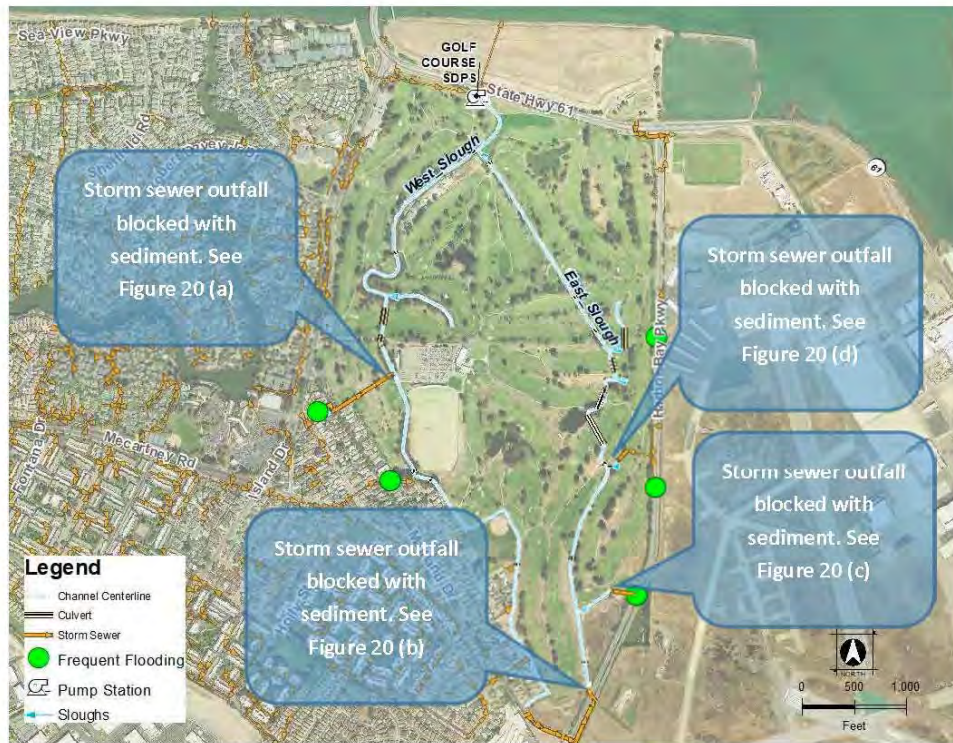
Figure 19 – Locations of Storm Sewers Outfalls Blocked with Sediment
