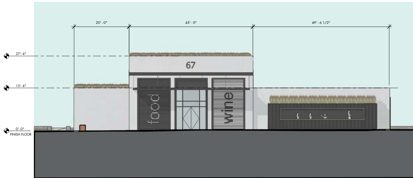
2 BUILDING 67 ELEVATION - SOUTH 3/32" = 1'-0"
