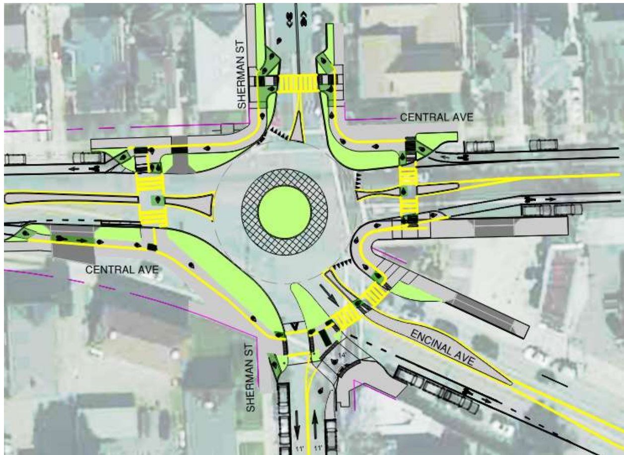
Figure 5: Recommended “Slip Lane” alternative
