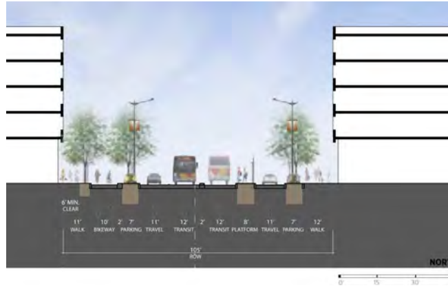
B. RALPH APPEZZATTO MEMORIAL PARKWAY - EAST 105' R.O.W. SECTION SECTION REVISED FROM PRECISE PLAN DOCUMENTS
