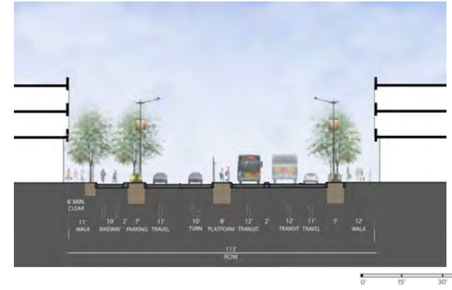
A. RALPH APPEZZATTO MEMORIAL PARKWAY EAST 113' R.O.W. SECTION AT MAIN STREET SECTION REVISED FROM PRECISE PLAN DOCUMENTS
