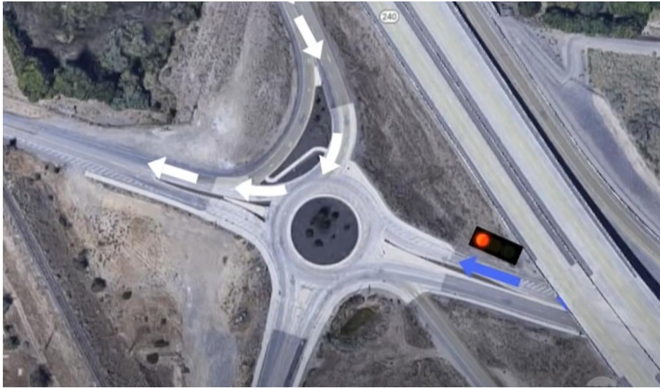
(a) Detectors installed on the north leg indicate a queue extending past a certain distance, triggering a red indication on the east leg
