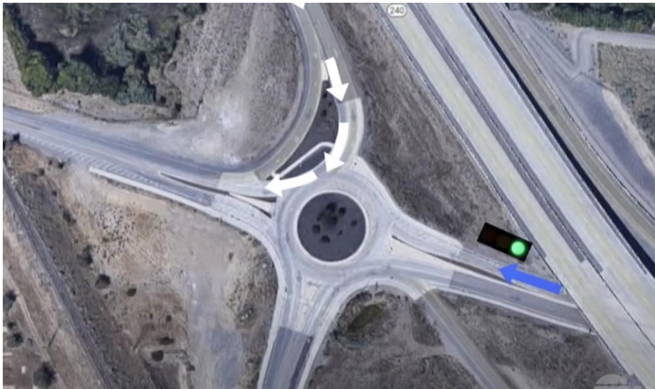
(b) The east leg can return to green or “pulse,” allowing one vehicle at a time, until the north leg queue has cleared.
