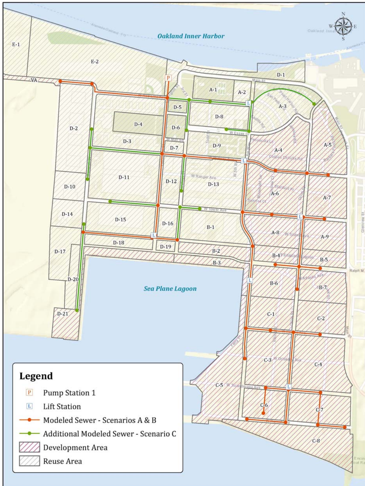
Figure 1: Alameda Point Proposed Sewer System - Modeled Network
