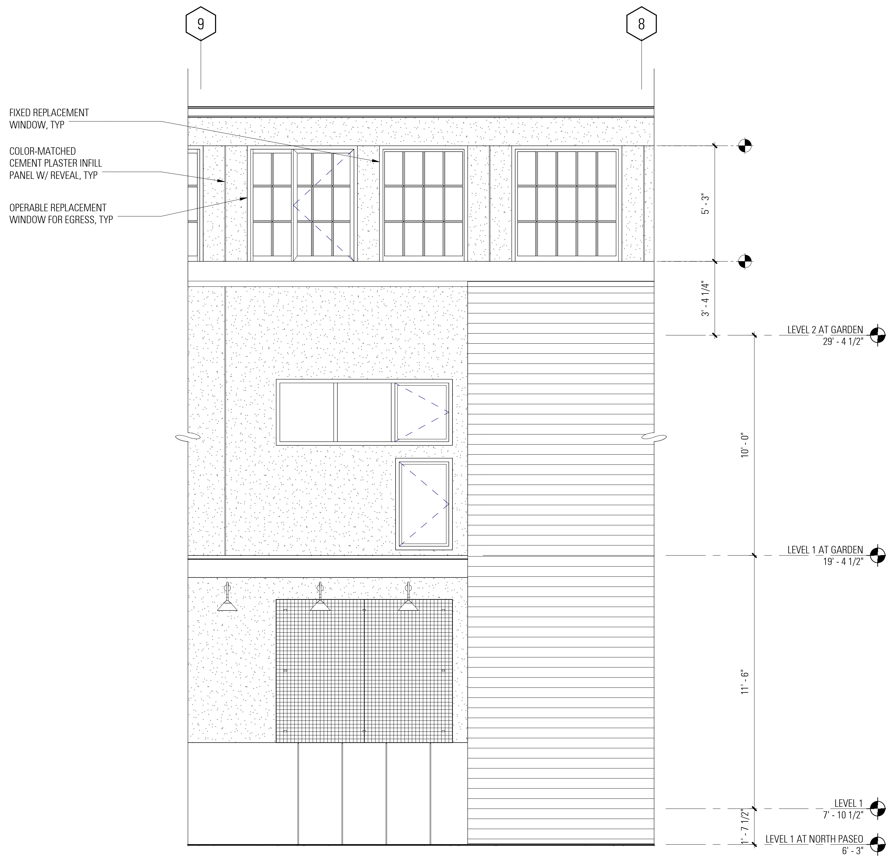
2 ENLARGED ELEVATION - TOWNHOMES AT PASEO W/ REPLACEMENT MONITOR WINDOWS RW-1 3/8" = 1'-0"
