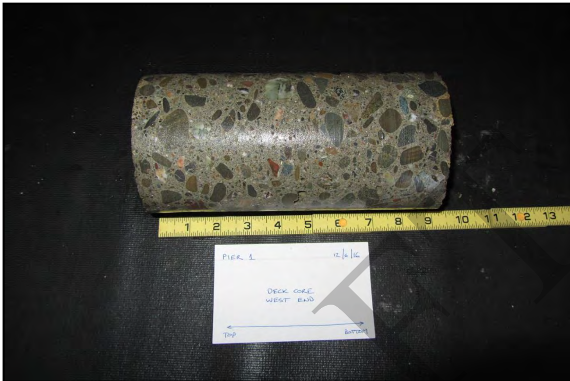
Photo 15: Concrete core sample taken from Pier 1 deck.
