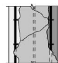
COMPLETE LOSS OF CONCRETE COVER DUE TO CORROSION OF REINFORCING STEEL
