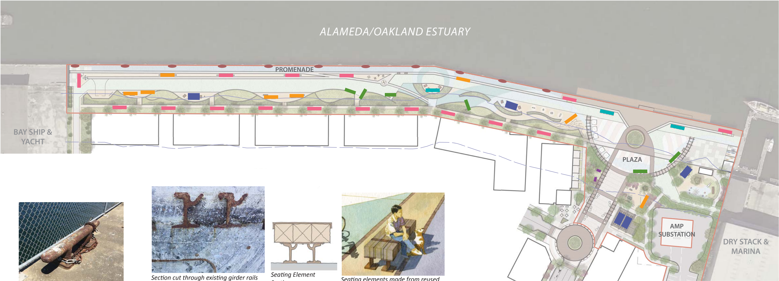
Seating elements made from reused girder rails and timber from the site
