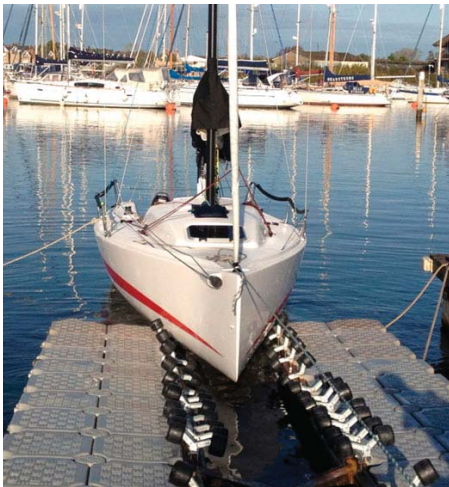
In-Slip Floating Dry Dock Example
