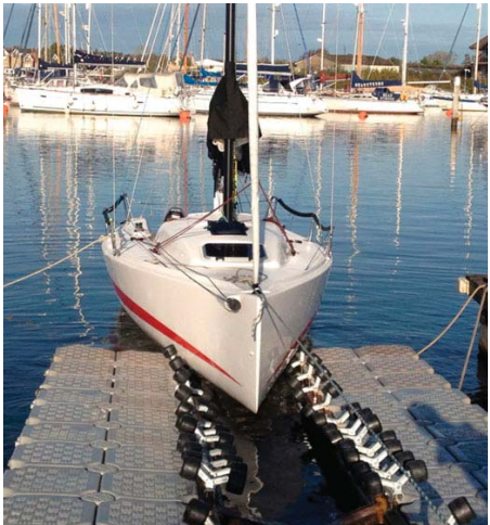
In-Slip Floating Dry Dock Example
