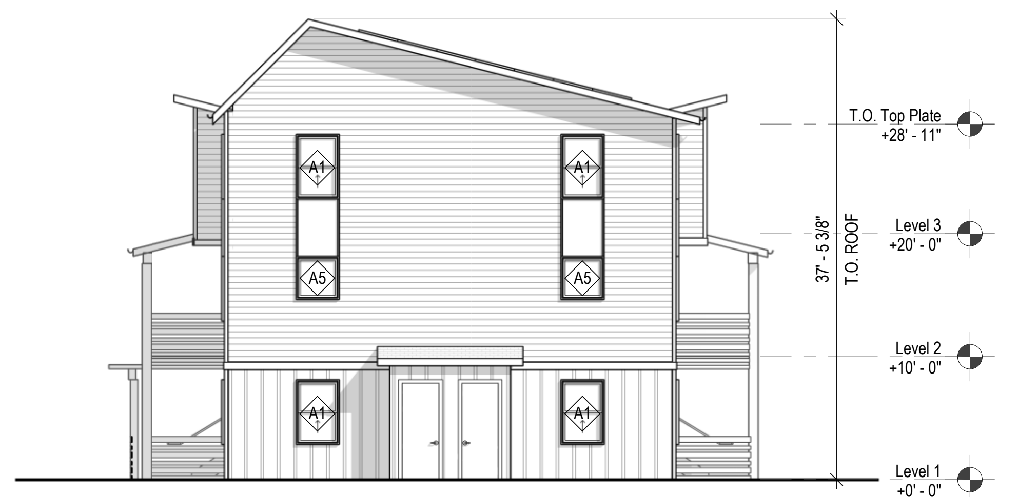
BUILDING 2 ELEVATION - WEST ④ 1/8" = 1'-0"
