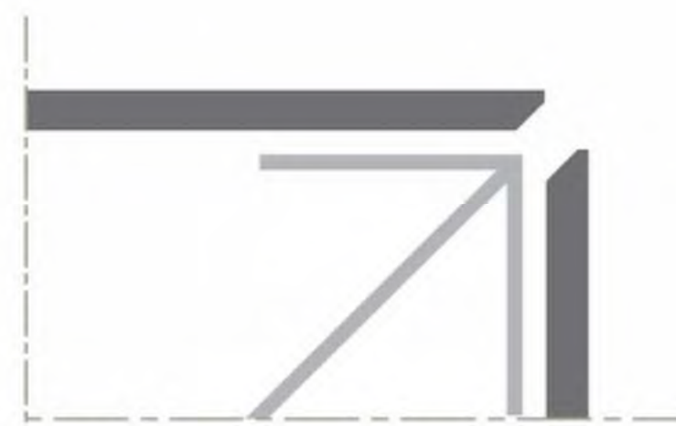
FACADE-FIBER CEMENT PANEL (TYP. CORNER)
